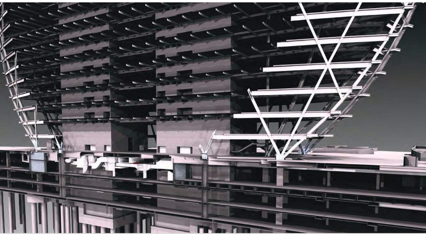
Figure 1-6 ALDAR Headquarters detailed construction model including steel and concrete detailing by Arup.
