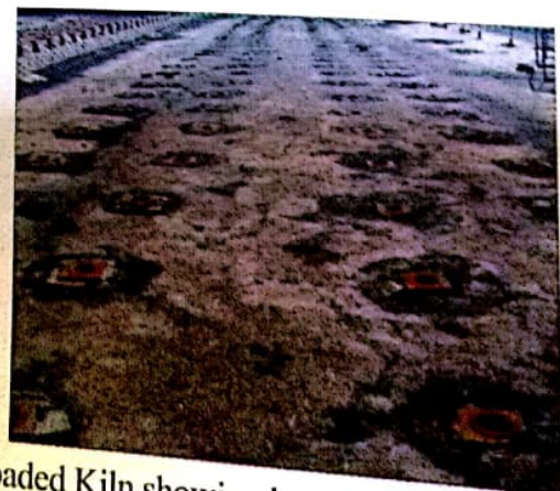
Stacking of Bricks-Note spacing for heat circulation
