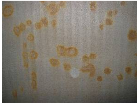
Figure 4.33. Trace of steel corrosion on a tank cover dome
