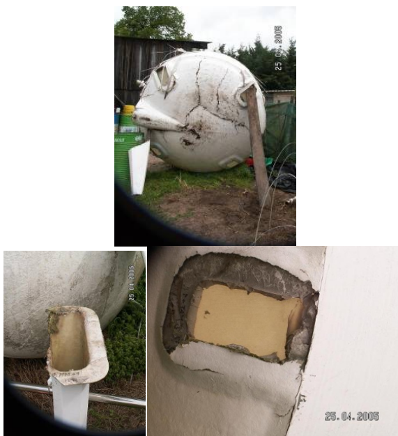
Figure 3.64. Pathology linked to a defect in characterization of stresses at the foot and a defect in the use of tissues
