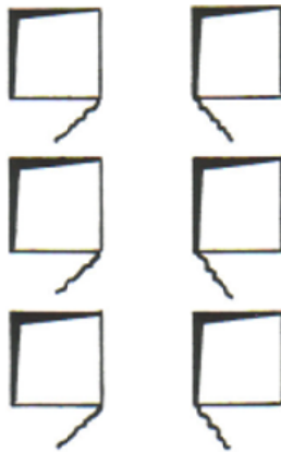
Figure 3.55. Cracks at 45° under different loads
