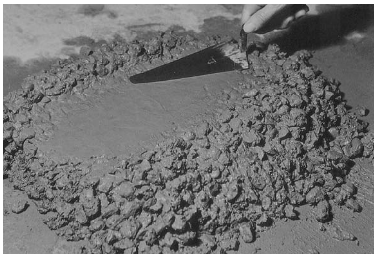
Plate 12b. Judging the quality of a concrete mix – a satisfactory mix. Photos from Concrete Materials and Practice by LJ Murdock, KM Brook, JD Dewar, 6th edition, Edward Arnold, 1991
