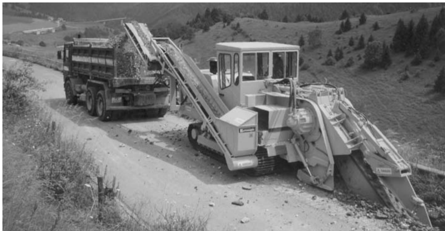
Plate 9a. A Mastenbrook 17/17 trenching machine with variable-offset heavy-duty cutting chain for trenches up to 0.6 m wide by 1.8 m depth. Larger machines are made. J. Mastenbrook & Co. Ltd, Boston, UK
