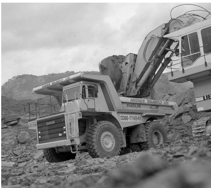
Plate 2b. A Euclid R60 522 kW dump truck, 36 m 3 heaped capacity. VME Construction Equipment GB Ltd, Duxford, Cambridge, UK
