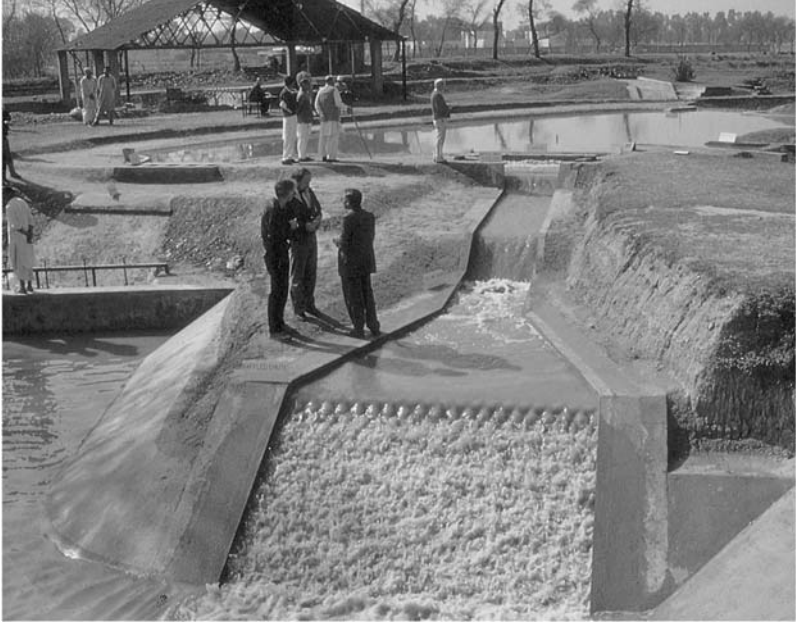
Plate 1a. The hydraulic model for the Ghazi Barotha Hydropower project, Pakistan, 1994
