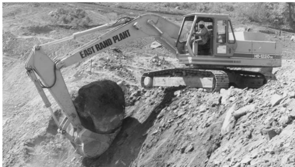
Plate 3b. A Kato 162 kW tracked excavator, with 1.6 m 3 bucket. ACP Holdings, Leicester, UK
