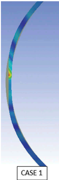
FIGURE 3.32 Deformation of ring stiffener at the collision zone.
