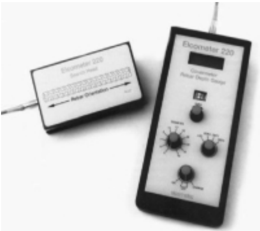
FIGURE 8.6 Shape of concrete cover thickness measurement machine.
