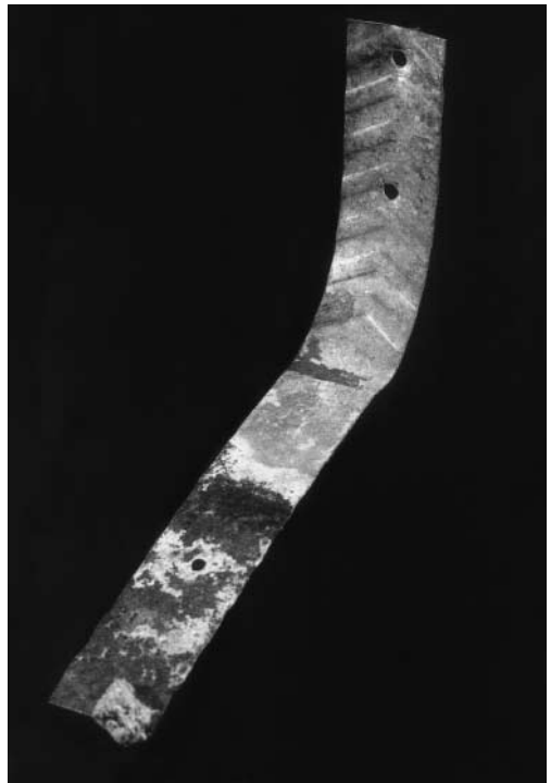
FIGURE 33.2 Corroded timber frame masonry wall tie showing both white rust ( \text{ZnO} ) and red rust ( \text{Fe}_2\text{O}_3 \cdot \text{H}_2\text{O} ).
