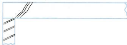
Fig. 4.3 Case of Complete Shear Failure.
