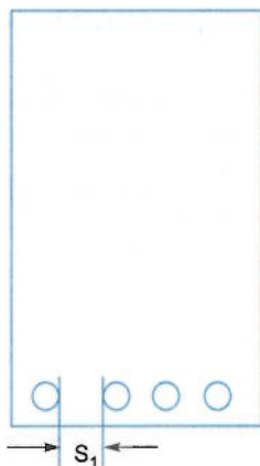
Fig. 5.12 Horizontal spacing between two bars.
