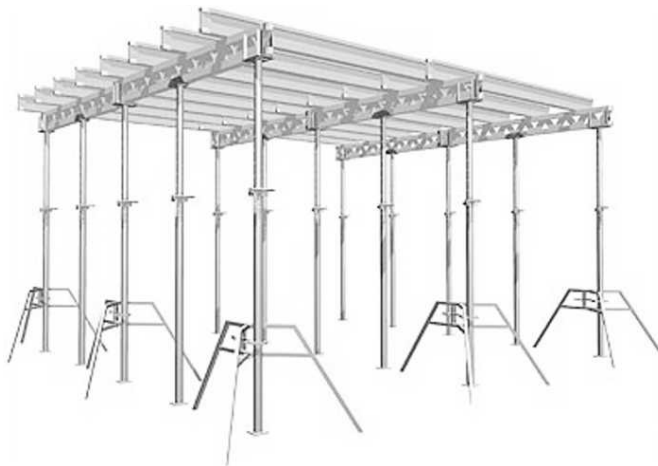
Figure 7.24 Multiflex Girder Slab Formwork (View showing Primary, Secondary Beams and Shores with Tripod) (Courtesy PERI).
