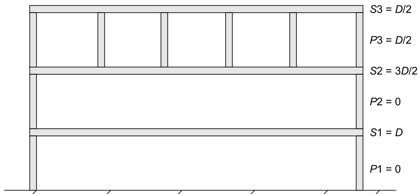
Figure 18.30 Removal of Shores Under Slab 2 on Day 26.
