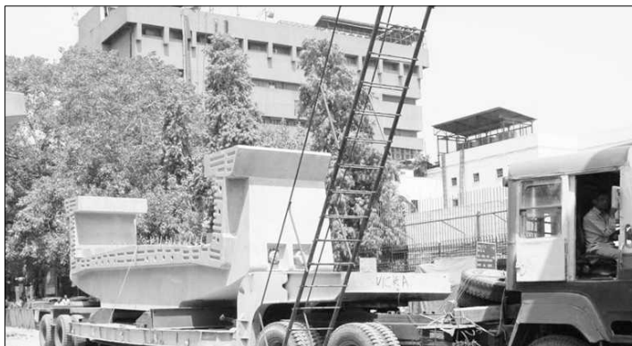
Figure 14.41 Low Bedded Trailer— Transportation of Segment to Site.
