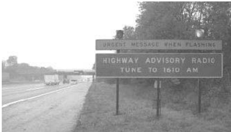
FIGURE 18.13 Highway advisory radio (HAR) effectively disseminate information to motorists at and near the incident scene.
