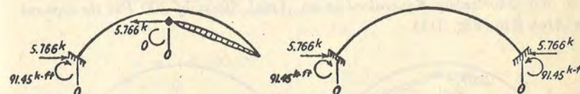
Induced reaction components due to a temperature rise of 50°F
