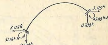
Induced reaction components due to rib shortening
