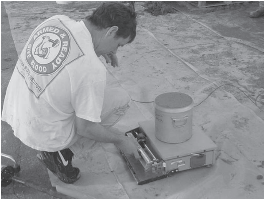
FIGURE A.33 Weighing concrete inside the container.
