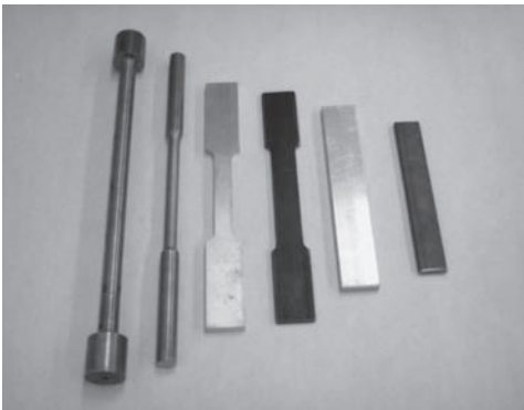
FIGURE 3.15 Tension test specimens with round and rectangular cross sections.
