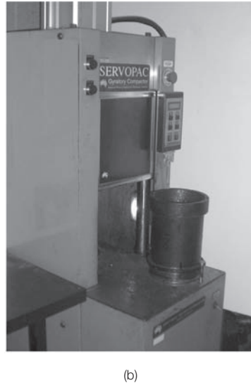
FIGURE 9.26 Superpave gyratory compactor. (Courtesy of Pavement Scientific International, Inc.)
