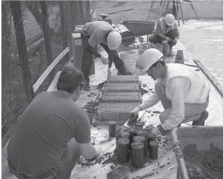
FIGURE A.36 Making concrete cylinders and beams.
