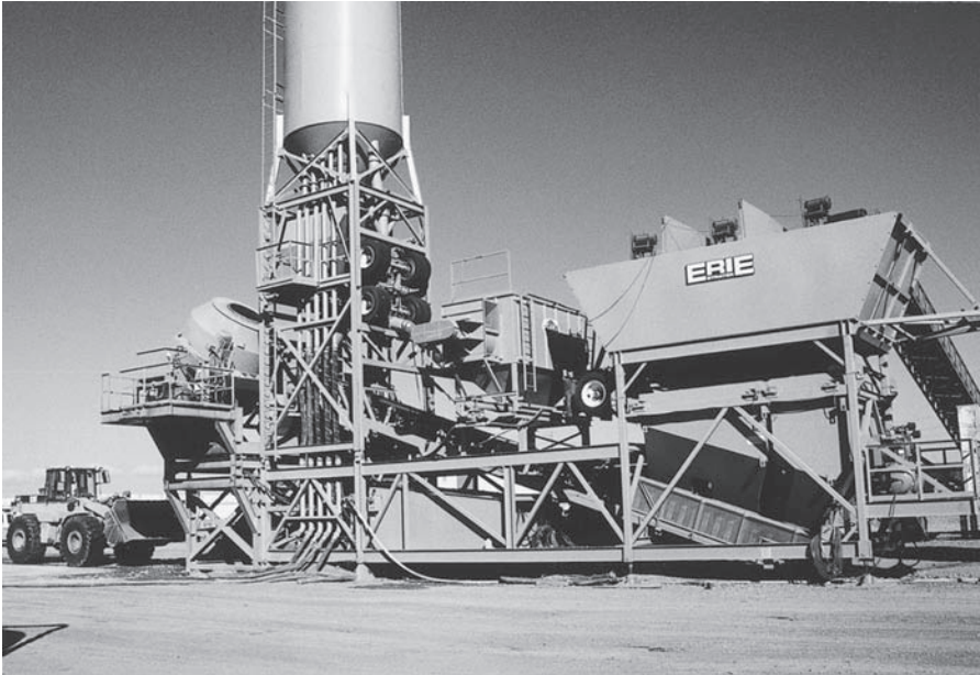
FIGURE 7.6 Mobile batcher mixer at the job site.
