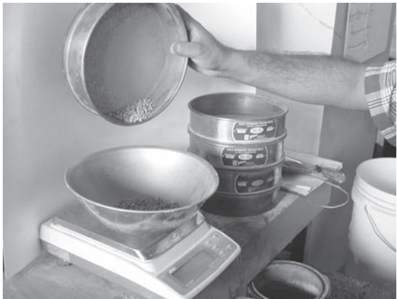
FIGURE A.23 Weighing aggregate retained in sieves.
