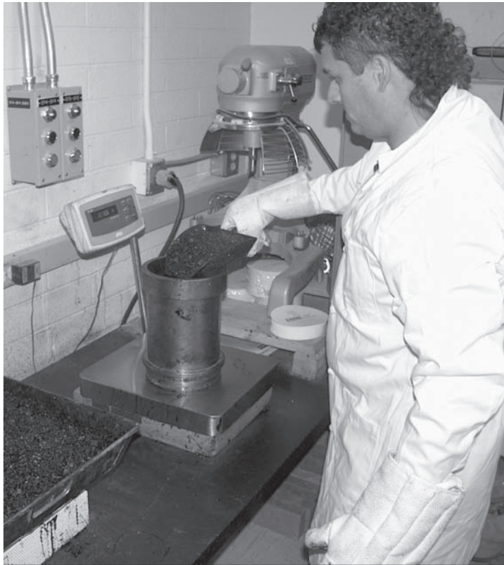
FIGURE A.57 Placing HMA in mold.
