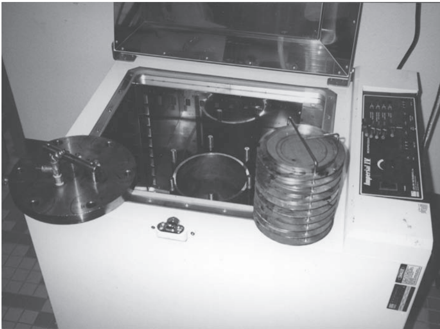
FIGURE 9.17 Pressure-aging vessel apparatus.
