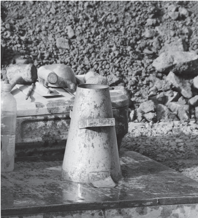
FIGURE 7.4 Slump test apparatus. (Fotolia/Bradlee Mauer)
