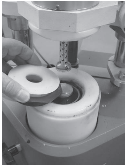
FIGURE A.54 Water bath for controlling specimen temperature during testing.
