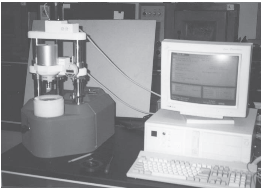
FIGURE 9.20 Dynamic shear rheometer apparatus. (Courtesy of FHWA)
