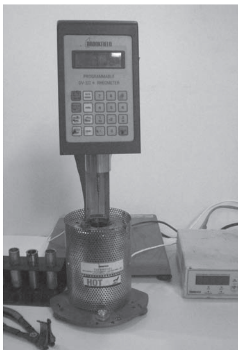
FIGURE 9.19 Rotational viscometer. (Courtesy of FHWA)
