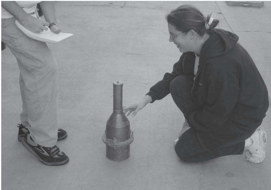
FIGURE A.35 Reading air meter.
