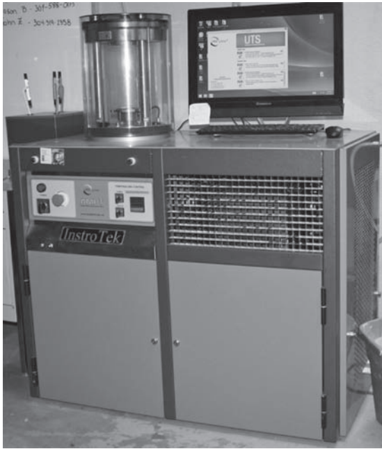
FIGURE 9.34 Asphalt Mixture Performance Tester.
