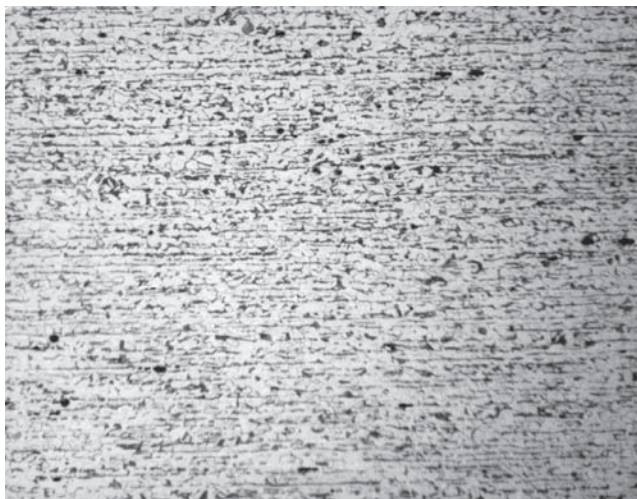
FIGURE 3.5 Optical photomicrograph of hot rolled mild steel plate (magnification: 50×).
