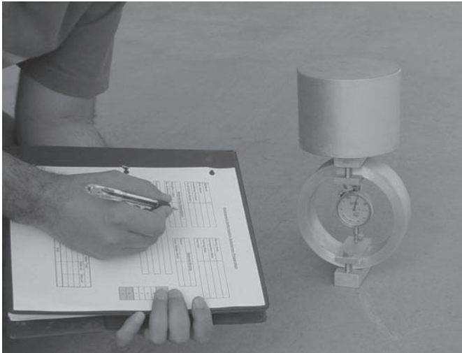
FIGURE A.3 Calibrating a proving ring using a known weight.
