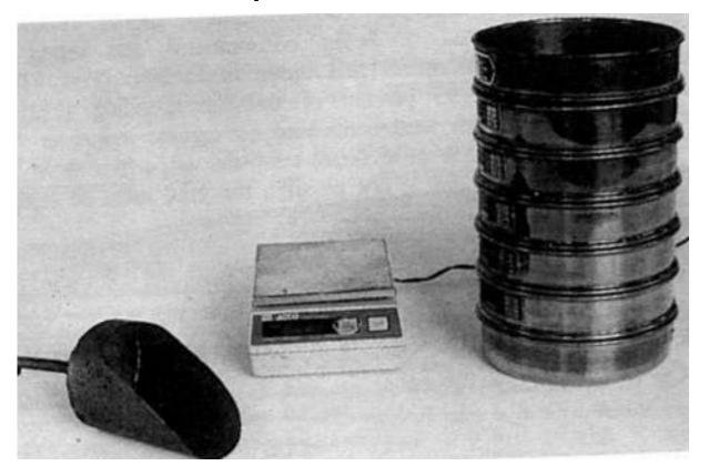
Equipments for Sieve Analysis Test on Aggregates
