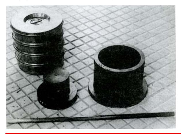
Equipments for Crushing Value Test on Aggregates
